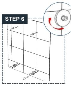
**STEP 6:** Insert the long screws through the mounting seats and then secure them into the plastic wall anchors with a electric drill. Place the decorative caps onto the mounting seats and tighten them.
